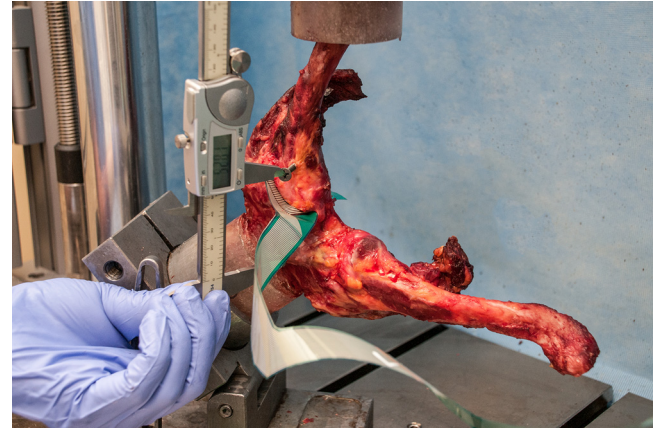
Figure 3. Measurement of the “native” distance between the marker screws with a digital caliper before testing of the joint pressure within the intact sternoclavicular joint.
