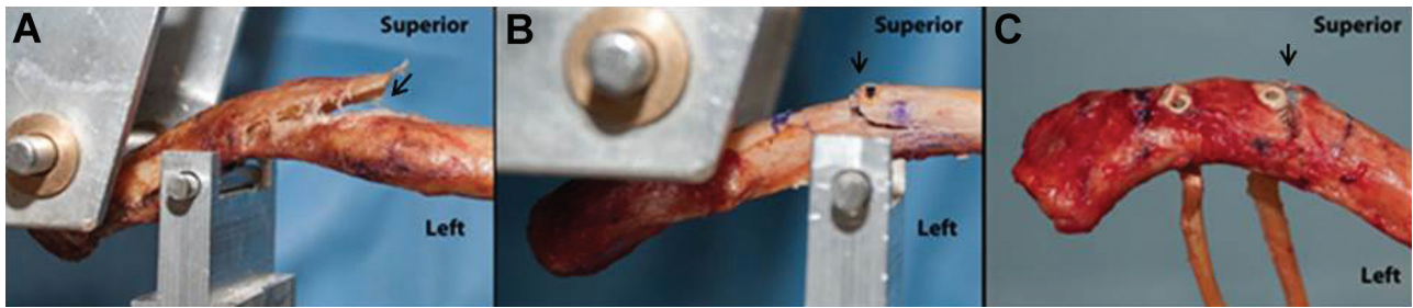
Figure 5. (A) Typical fracture pattern of intact clavicles, as well as after (B) cortical fixation button reconstruction and (C) tendon graft reconstruction. Arrows indicate the fracture site.
