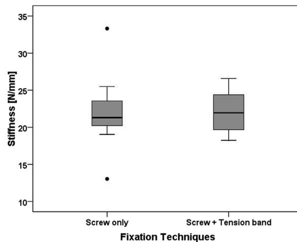
**Figure 4** Box plot comparing the stiffness of the simulated os acromiale fixed with screws only (SO group) vs. screws in combination with a tension band (TB group). There were no significant differences between both groups. Both *dots* represent outliers in the SO group with stiffness of 13.0 N/mm and 33.3 N/mm.
