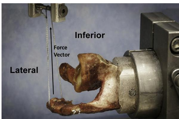
**Figure 1** Biomechanical test setup. A high-strength suture tape (FiberTape; Arthrex, Naples, FL, USA) was inserted into the acromion 1 cm from the anterior tip. The 2 ends were tied around a 10-cm-diameter cylinder and looped around a rod fixed to the actuator of the tensile testing machine. The testing jig was positioned so the pull vector was perpendicular to the surface of the acromion.
