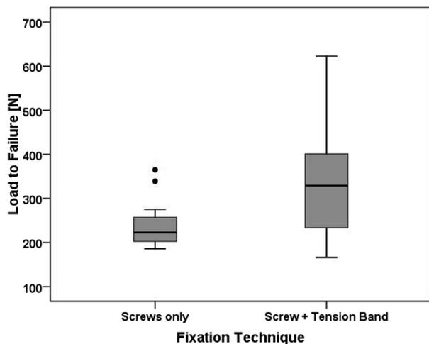
**Figure 3** Box plot comparing the ultimate failure loads of the simulated os acromiale fixed with screws only (SO group) vs. screws in combination with a tension band (TB group). The TB group failed at significantly higher loads ( $P = .01$ ) than the SO group. *Dots* represent positive outliers in the SO group with ultimate failure loads of 339 N and 365 N.
