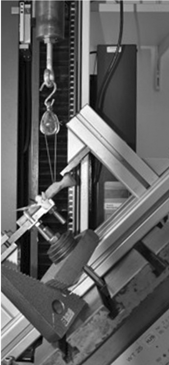
Figure 2. Setup for biomechanical testing on servohydraulic machine.
