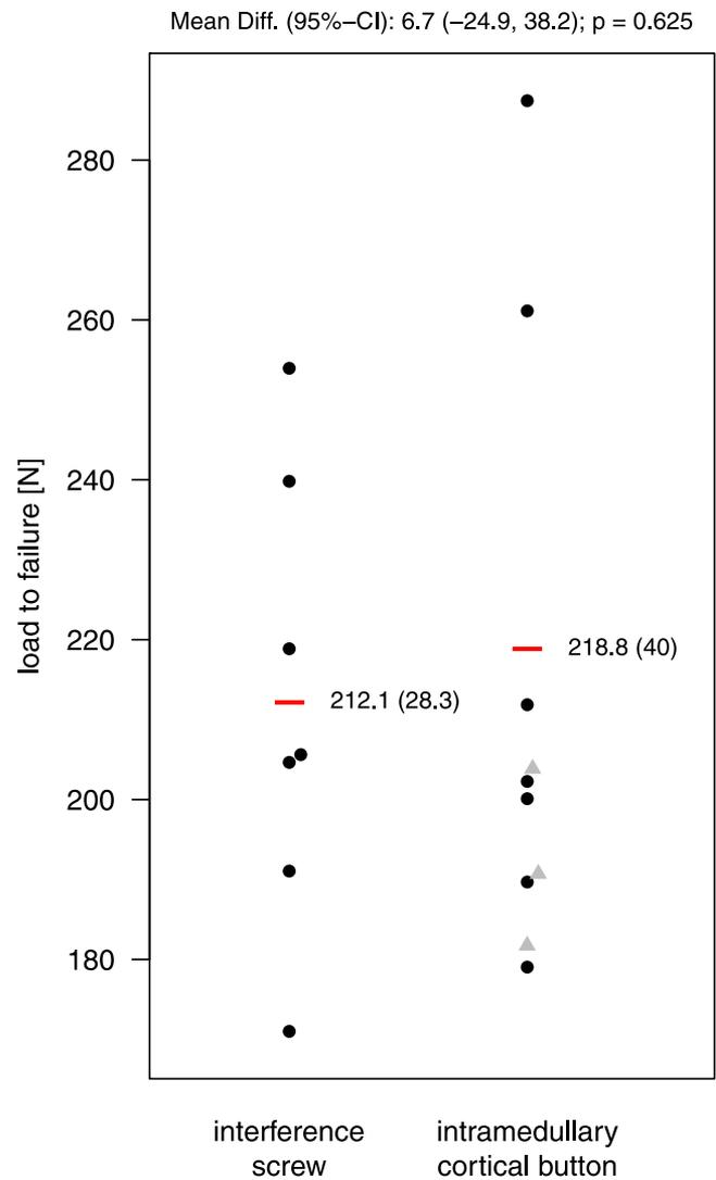
**Fig 4.** Scatter plot of load to failure with mean and standard deviation of each repair group. Mean difference (Diff), respective 95% confidence interval (CI), and  $P$  value are also presented. The measured values in the intramedullary cortical button group, which correspond to the 3 failures in the interference screw group, are presented (triangles) for the sake of completeness. They were not included in the analysis.
