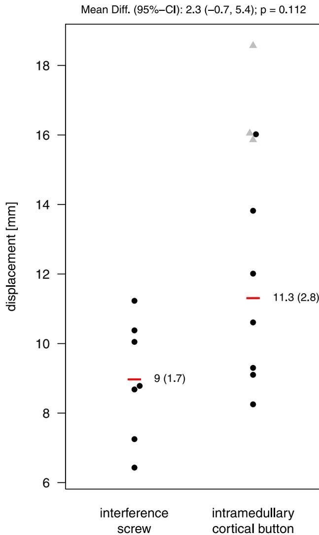
**Fig 3.** Scatter plot of displacement after cyclic loading with mean and standard deviation of each repair group. Mean difference (Diff), respective 95% confidence interval (CI), and  $P$  value are also presented. The measured values in the intramedullary cortical button group, which correspond to the 3 failures in the interference screw group, are presented (triangles) for the sake of completeness. They were not included in the analysis.
