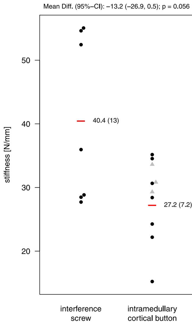
**Fig 5.** Scatter plot of stiffness with mean and standard deviation of each repair group. Mean difference (Diff), respective 95% confidence interval (CI), and  $P$  value are also presented. The measured values in the intramedullary cortical button group, which correspond to the 3 failures in the interference screw group, are presented (triangles) for the sake of completeness. They were not included in the analysis.
