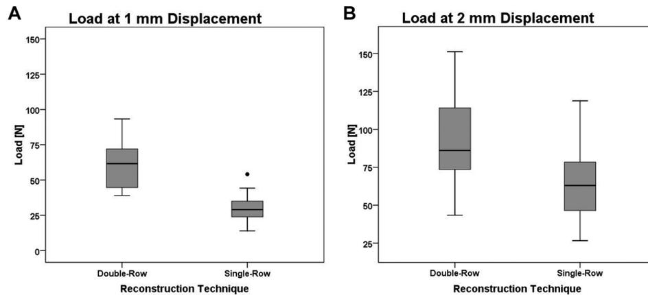
**Figure 5.** Box plots displaying loads to displace the fracture defect by (A) 1 mm and (B) 2 mm. The double-row repair required significantly higher loads to achieve 1 mm ( $P = .001$ ) and 2 mm of displacement ( $P = .004$ ) compared with the single-row repair.
