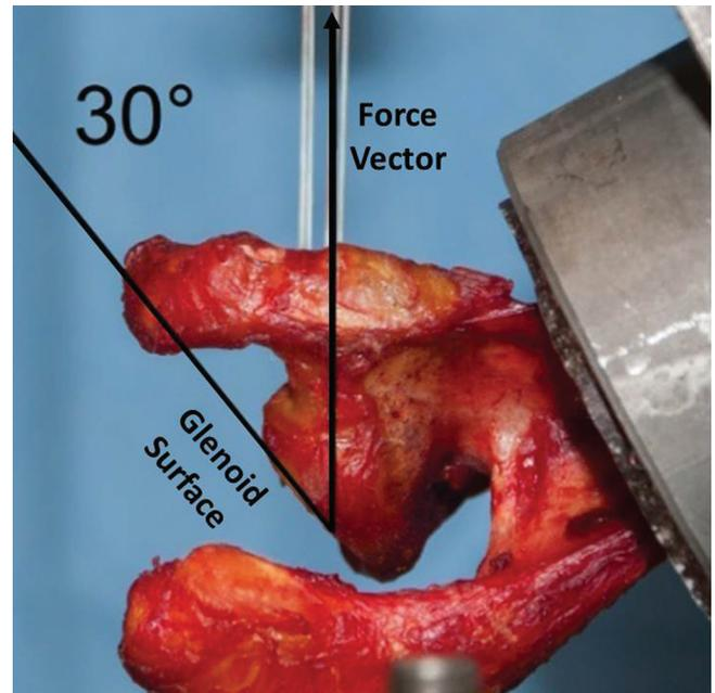
**Figure 4.** Testing setup: The specimen was fixed in a custom jig with the glenoid face oriented to create a loading vector 30° medial to the anterior-posterior plane.
