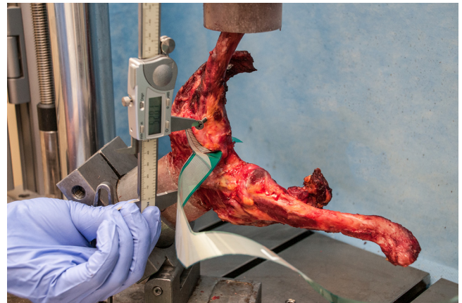
Figure 3. Measurement of the "native" distance between the marker screws with a digital caliper before testing of the joint pressure within the intact sternoclavicular joint.
