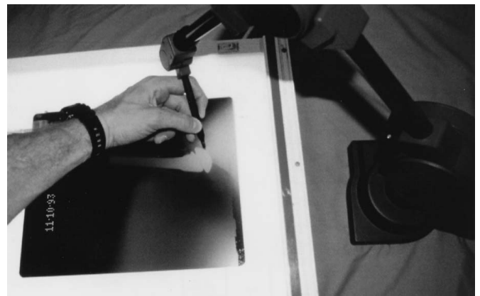
Fig 1. The Microscribe 3-DX digitizing device consists of a serially articulated arm with a terminal stylus for accurate measurement. The base contains a reference coordinate system within which a series of Cartesian coordinates can be defined. The reported accuracy for this device is 0.23 mm.
