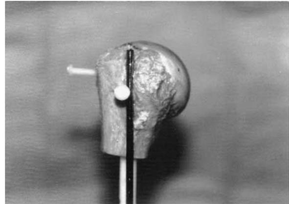
**Figure 2** Photograph of specimen in custom jig. Specimens were fixed to the polyethylene post with 2 polyethylene screws at 90° to each other in order to prevent rotation and migration.
