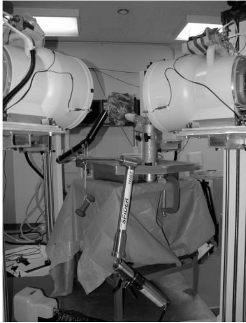
Figure 4. Testing setup overview. The cadaveric shoulder was clamped on a commercial rig with the humerus mounted in PVC tubes that allows attachment to a pneumatic arm holder. This setup was placed in the biplane fluoroscopy system.
